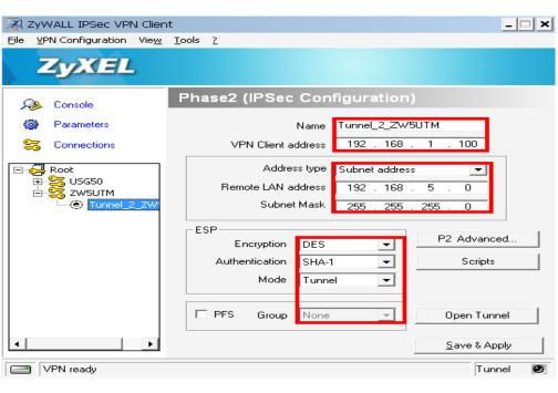
Step 8. Configure the phase-2 parameters.
