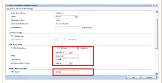
Step 9. After the configuration is done, click **Activate** to enable the rule. And then click Connect button to enable the 3G connection.
