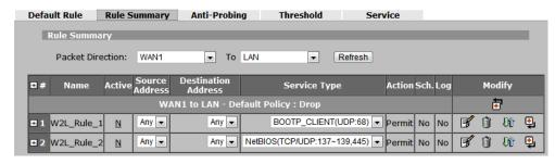
Step 6. Configure the firewall rule to enable the FTP service to pass from WAN1 to LAN.
