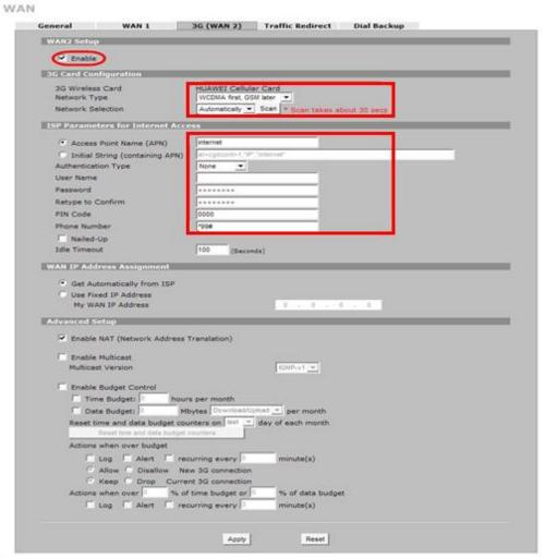
Step 8. Fill in the 3G connection parameters:
