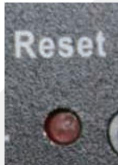
Plug the power in and make sure the camera has fully booted. Press the reset button for 6 seconds.
