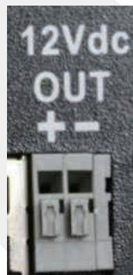
When using the 12V DC in-box port, connect the device with the video server by inserting the positive/negative wire into the appropriate hole.
